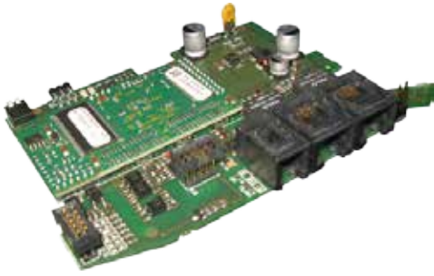
Figura 35 Port2: Modbus RTU / Ethernet IP or Modbus RTU/EtherCAT or Modbus RTU / ProfiNET Interfaces
