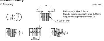
When mounting the coupling to the encoder shaft, if there is combined misalignment (parallel, angula misalignment) between rotating encoder shaft and mate shaft, it may cause encoder and coupling's life cycle to
