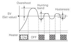
As like above picture, the control value is up and down by set value, it is called Hunting. And Overshoot is occurred at initial point when just
